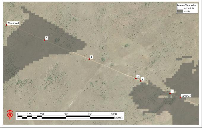
The shaded areas indicate the areas that would be targeted by the radio signal emitted by the jamming signal generator.
