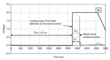
Fig. 9. The pressure history and optical sensor output in voltage for Event 2.
