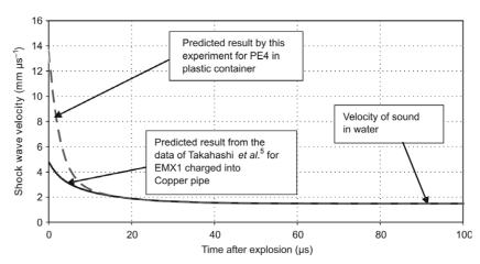
Fig. 14. A plot of the shock wave velocities in the near field of an underwater explosion for two different compositions of explosives.
