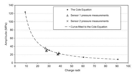
Fig. 8. The amplitude of the pressure (MPa) measured in this study, versus the standoff distance (charge radii), compared to that obtained by the equation given by Cole.<sup>2</sup>
