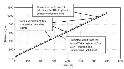
**Fig. 13.** A plot of the distance travelled by the shock wave versus the time taken for that distance to be travelled, obtained by measurement in this study and by the equation of Takahashi *et al.*<sup>5</sup>
