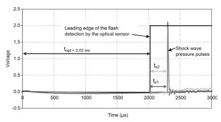
Fig. 11. The pressure history and optical sensor output in voltage for Event 4.
