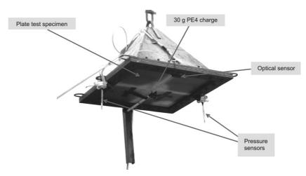
Fig. 6. The position of the optical sensor, relative to the pressure sensors, for Events 4 and 5.
