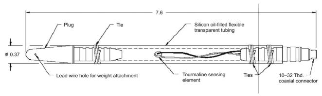
Fig. 7. Schematic diagram of pressure sensor.
