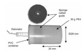
$\textbf{Fig. 3}. The components and assembly of the 30-g \, PE4 \, charge \, used \, in \, this \, study.$
