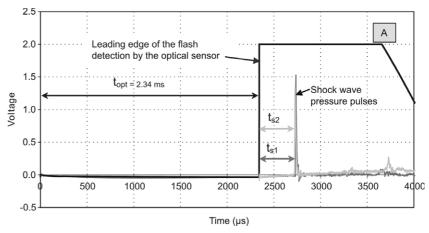
Fig. 10. The pressure history and optical sensor output in voltage for Event 3.
