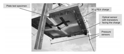
Fig. 5. The position of the optical sensor mounted on the frame, relative to the explosive charge and the pressure sensors, for Events 2 and 3.
