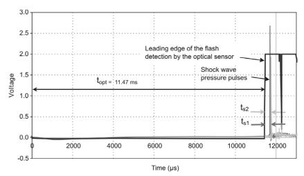
$\textbf{Fig. 12}. \ \textbf{The pressure history and optical sensor output in voltage for Event 5}.$
